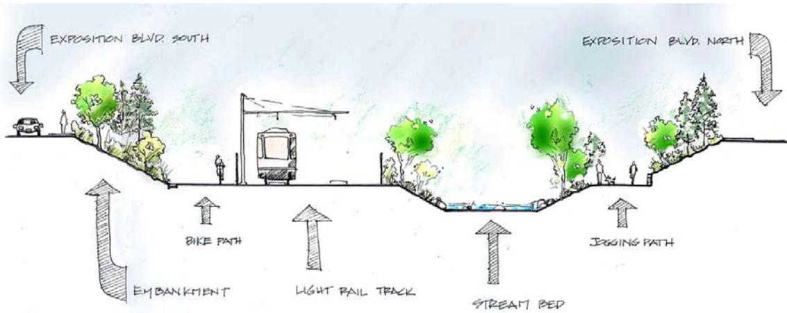
Use of the wide right-of-way for this configuration of light rail tracks in a shallow, soil-lined trench with short underpass structure may be **no more costly**, and is certainly **much less visually impacting** than a conventional overpass with retained-fill ramps edged with soundwalls. **Water quality funds** may complement transit funds for this.
